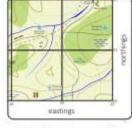
then the vertical axis, called the northing, from south to north, until they meet at the bottom left-hand corner of the square you want to reference. The easting followed by the northing makes a four-figure grid reference. The four-figure grid reference for the square containing Shawdale Cathedral is 18 00.
