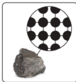
Solid metals are thermal conductors because their strong, metallic lattice bonds transfer heat.
