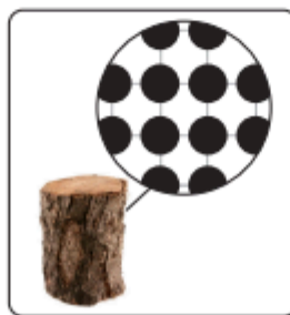
Other solids do not have strong, metallic lattice bonds so they do not conduct heat.
